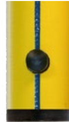
Roll Pins use a 1/8" Drill Bit
