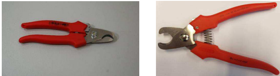
Figure 3.2 TE recommended Knipex cut-tool, 95 05 165 (or equivalent)
