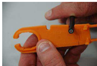
Figure 4.3 – determine if cable-outer-diameter is within min. and max. range with delatching-tool PN 2342988-1. Use the min. and max. cable openings on the tool to check if your cable is within the range yes or no.
