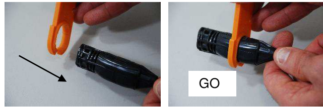
Figure 5.4 – Control termination with TE delatching-tool PN 2342988-1 (figure 7.1)
