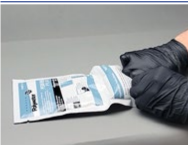
Burst primary seal
