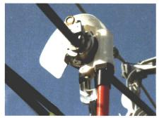
STEP # 6. Before the tool is placed on the conductor make sure the blade set ring is pushed all the way in. Turn the handle counter clockwise to open the tool, placing the tool on the conductor against the tool stop. While pushing the tool up slightly, seat the cable in the lower halve of the jaw. Begin turning the handle clockwise closing the bushing around the cable until it is fully closed, an audible click will be heard.
