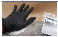
**8.** Apply constant pressure to this Putty patch with the palm of the hand for 2–3 minutes until material feels firm. Save a piece of the mixed putty to use as an indicator to tell when the putty is hard. For the best long-term seal, limit quantity of Putty.
