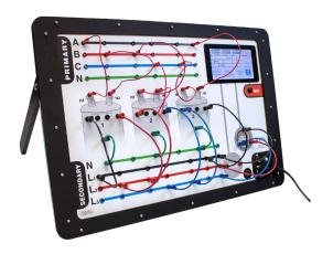
The Load-Trainer™ II provides an immersive learning experience for transformer banking and 3 phase simulation. Real-time information is displayed when the 'TEST' button is pressed.
