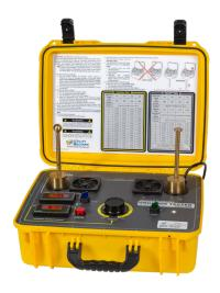
The Grounds Tester is portable, compact and utilizes a voltage (AC) at high current to measure voltage drop across personal grounding equipment. Pass/fail determinations are made by comparing the voltage drop to convenient charts in the manual and on the case lid.
