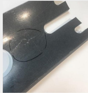
Figure 2.13.4 – Circled break point area image
